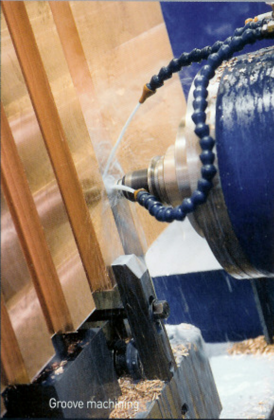
Fully machined copper Stave
