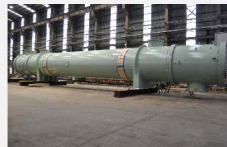
CCW Heat Exchanger
