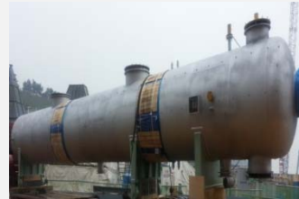
L.P. Feed Water Heater
