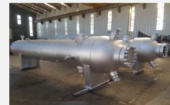
Fuel Gas Heater
