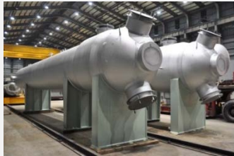
H.P. Feed Water Heater
