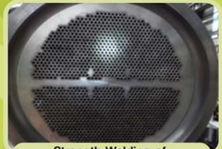
Strength Welding of Tube to tubesheet
