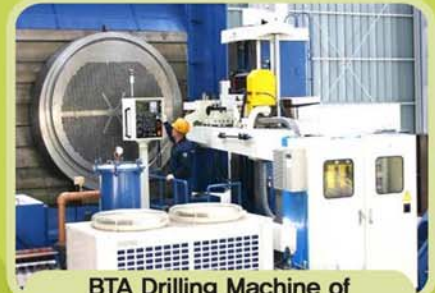
BTA Drilling Machine of 40"(1016mm) Tubesheet
