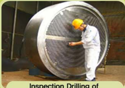
Inspection Drilling of 21.5"(545mm) tubesheet
